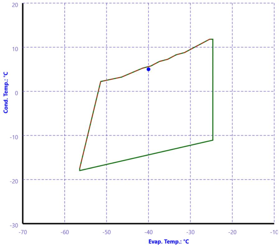
Figure 4.4: Field of operation for GEA Grasse 35HP using R744[24]
