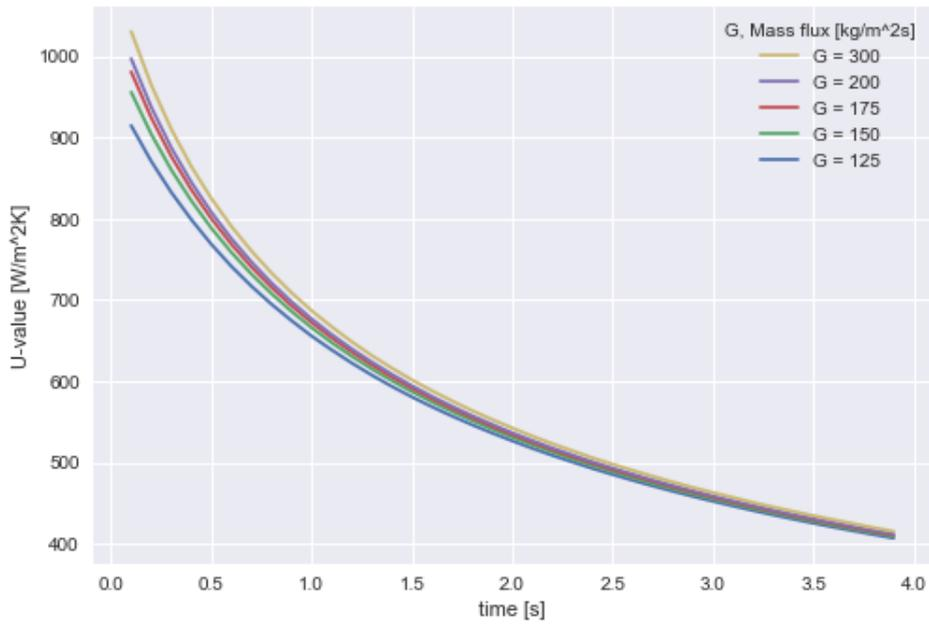
Figure 5.5: Average U-value of ice-formation, coiled configuration
