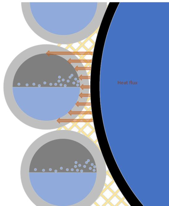
Figure 4.2: Vertical pipes configuration, seen from above
