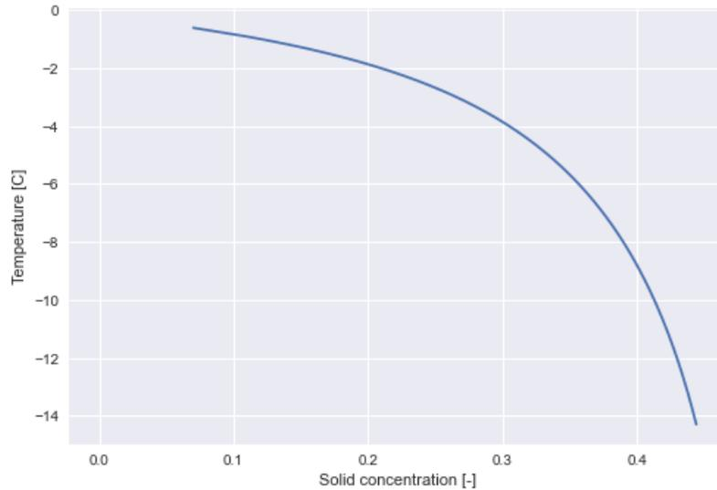
Figure 2.6: Freezing depression of the FPH mixture [7]
