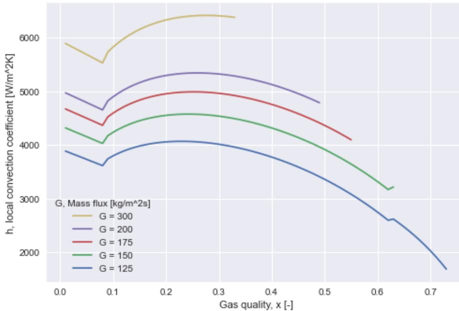
Figure 5.1: Initial CO<sub>2</sub> convection coefficient with increasing gas quality, coiled configuration
