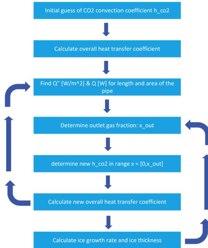
Figure 4.3: Algorithm CO<sub>2</sub> convection coefficient
