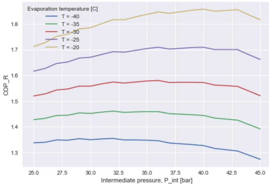
Figure 5.15:  $COP_R$  with varying  $P_{int}$  for a range of evaporation temperatures
