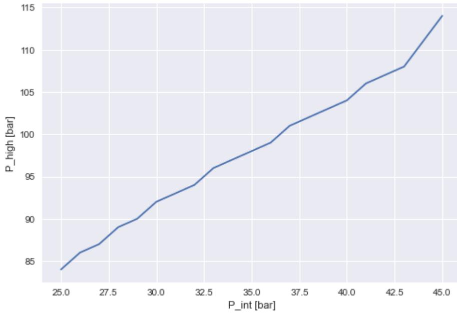
Figure 5.14: Minimum high side pressure vs intermediate pressure
