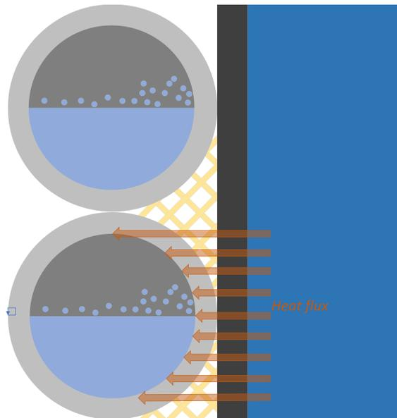
Figure 4.1: Proposed evaporator design w/coiled pipes
