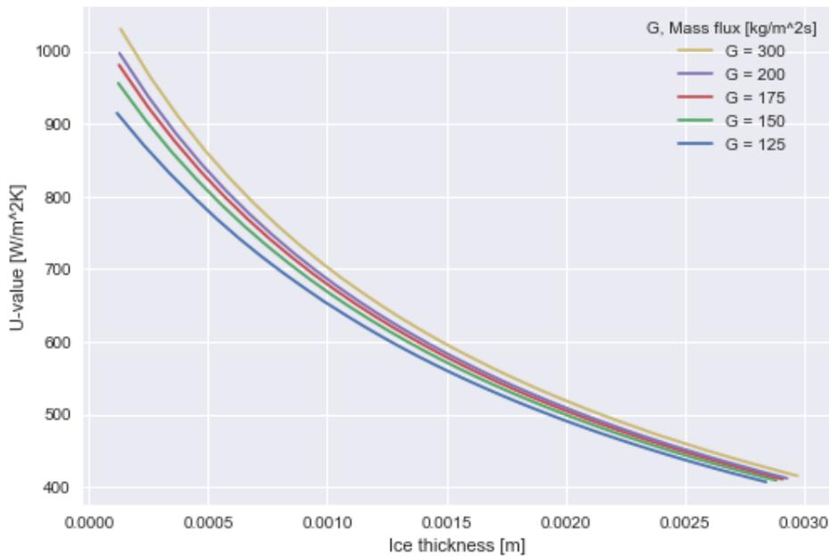
Figure 5.6: U-value vs Ice thickness, coiled configuration
