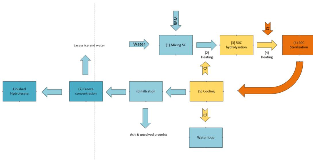
Figure 3.1: Flow sheet of the hydrolysate proces
