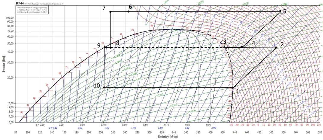
Figure 3.4: CASE 1 example visualized in log P-h diagram
