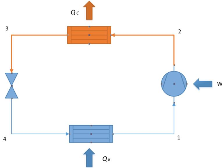
Figure 2.1: Illustration of a simple refrigeration cycle
