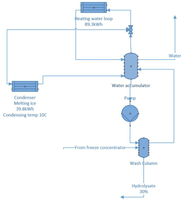
Figure 3.2: Illustration of the proposed water-loop
