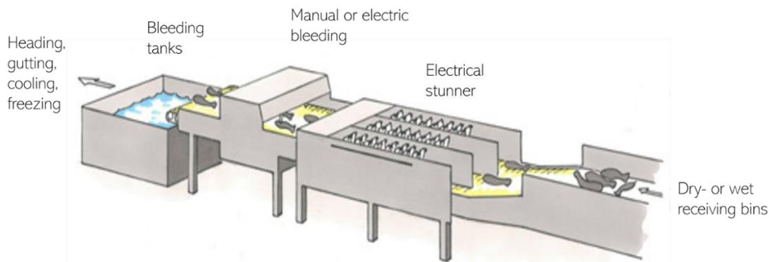
Figure 10. A generalized on-board processing line. Illustration: Mats Heide, SINTEF Ocean (Digre et al., 2015).
