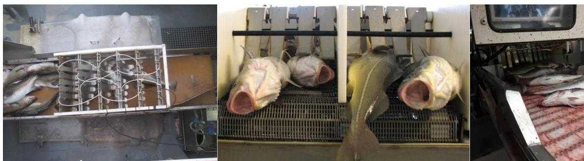
Figure 12. Electrical stunning of fish on board. Photo: SINTEF Ocean. (Erikson et al., 2014)
