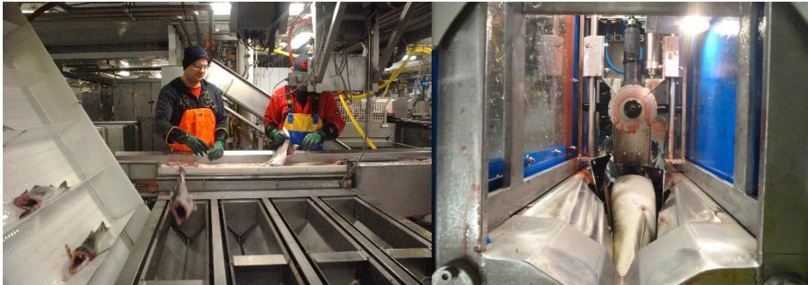
**Figure 13.** Both electrical and manual heading are used on board Norwegian fishing vessels. Some vessels only bleed and gut the fish (not removing the head). Photo: SINTEF Ocean.
