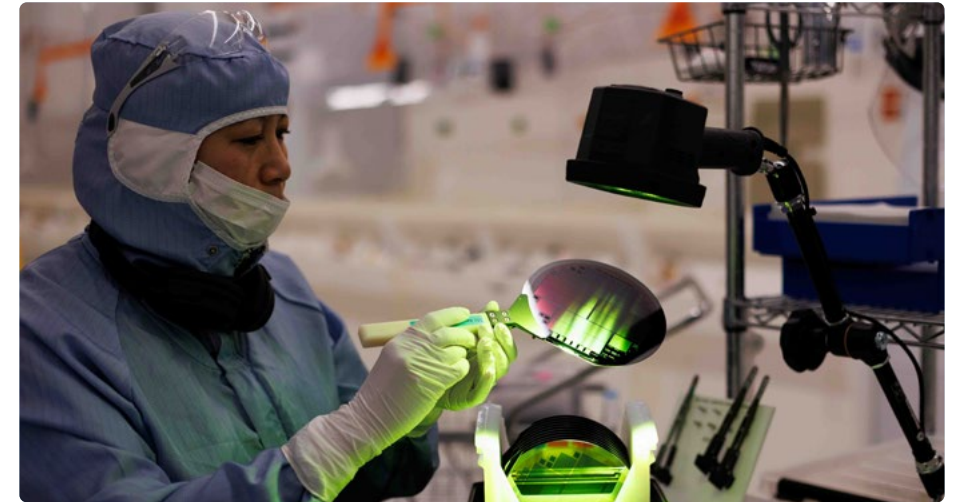
Silicon wafers under the microscope: Senior Engineer Leny Nazareno inspects silicon wafers for particles and pattern defects. The powerful green light is monochromatic (single-coloured), making even small particles and pattern defects visible without a microscope.
