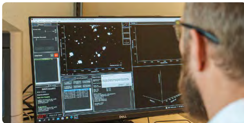
Researcher Andreas Åslund is researching nanotechnology to improve drug delivery to patients. Here he is analysing the size of nanoparticles that contain pharmaceuticals using Nanoparticle Tracking Analysis (NTA). Photo: Smidesang & Lyng/SINTEF
