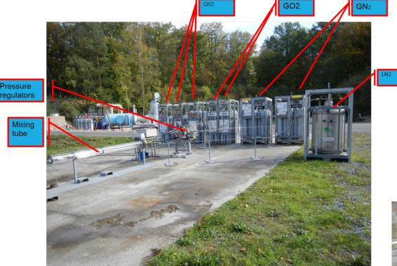
Performance: •4% to 80% H<sub>2</sub> •Ambient to -150°C •Ambient pressure
