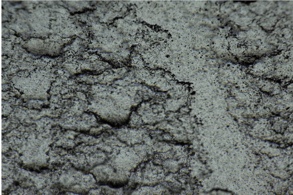
Sample from S3 04-21/08/2020 (extreme soiling over 2-week period)
