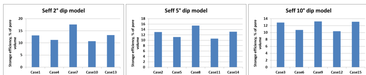
Figure 4 Storage efficiency as percent pore volume occupied by CO 2 for the different simulated cases.
