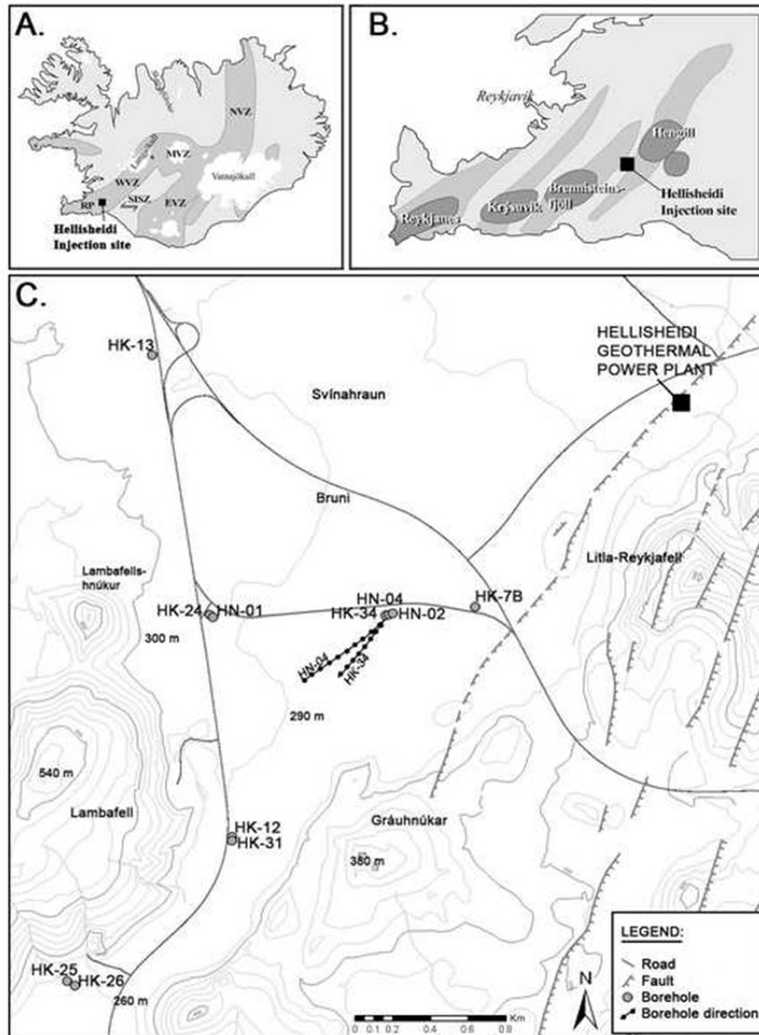
**Figure 8.3:** Map of the CO<sub>2</sub> injection site in Hellisheidi, SW-Iceland. The CarbFix wells are shown as labelled gray dots. Mapped bedrock faults are located towards east and are part of the Hengill fissure swarm. The cross section shown in Figs. 2 and 4 is marked A-A' (from: Alfredsson et al. 2012).
