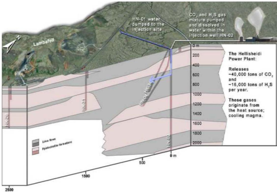
**Figure 8.4:** Geological cross section of the injection site in Hellisheidi. The  $\text{CO}_2$ – $\text{H}_2\text{S}$  gas mixture will be separated from other geothermal gases at the power plant, and pumped towards the injection site and mixed with water from well HN-1 within the injection well HN-2. The gas charged waters enters the basaltic formations as single phase; water phase (Alfredsson et al. 2012).
