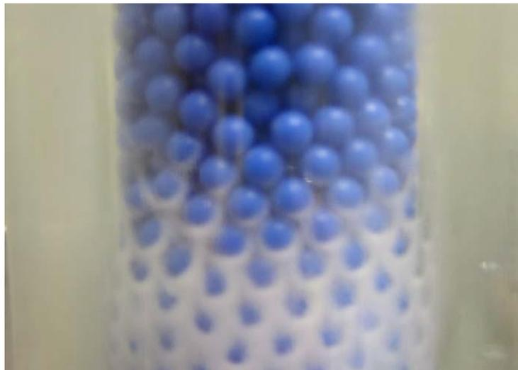
**Figure 2.21** CO<sub>2</sub> solidification on pre-cooled packed bed. Facsimile from<sup>51</sup>.
