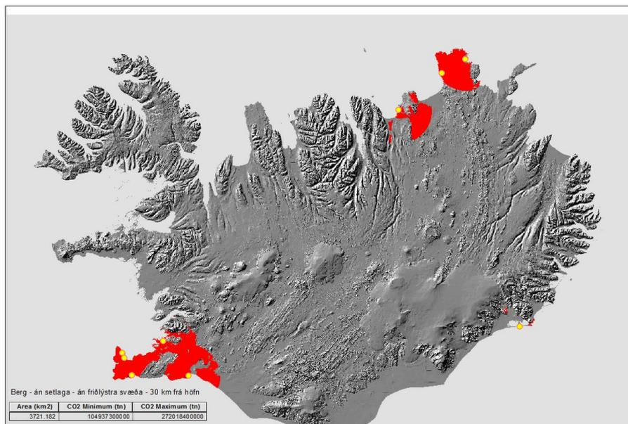
**Fig 4.** Theoretical area feasible for CO<sub>2</sub> mineral storage in Iceland: Basaltic formations younger than 0.8 M yr. within a 30 km radius of a large-scale harbor (marked with yellow dots).
