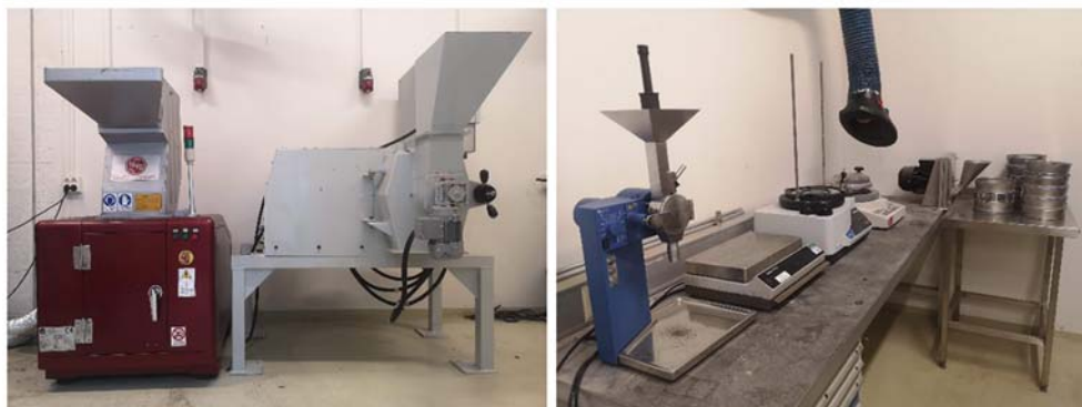
Figure 5 Fuel preparation facility showing the tabletop equipment for milling and sieving to the left and the large-scale mill and pellet-press machine to the right
