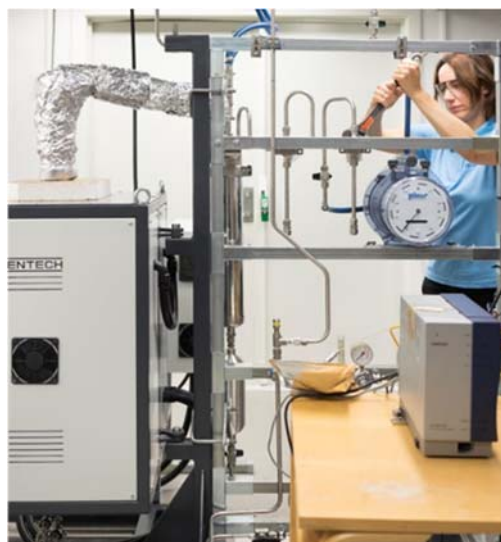
Figure 1 The pyrolysis and carbonisation reactor
