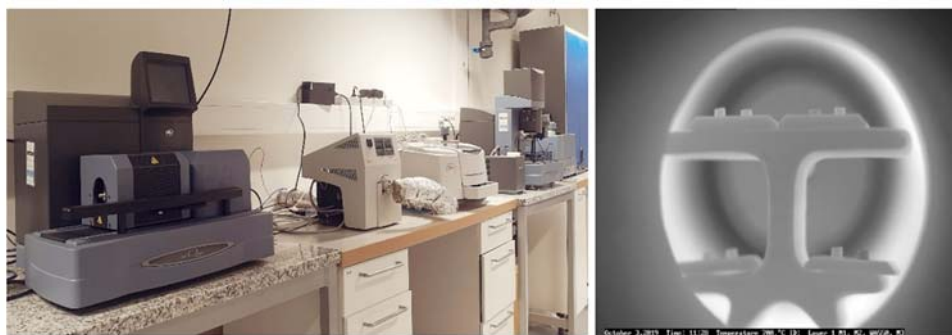
Figure 6 Characterisation equipment at SINTEF Energy laboratories (left) and the ash melting microscope (right)
