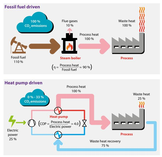
Figure 2: Comparison of fossil fuel driven and heat pump driven industrial process schemes.
