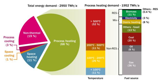
**Figure 1:** Breakdown of the final energy demand in European industry by broad application (left) and process heating demand by temperature level (centre) and energy source (right) (RES = renewable energy sources) Data source: <sup>1,3</sup>
