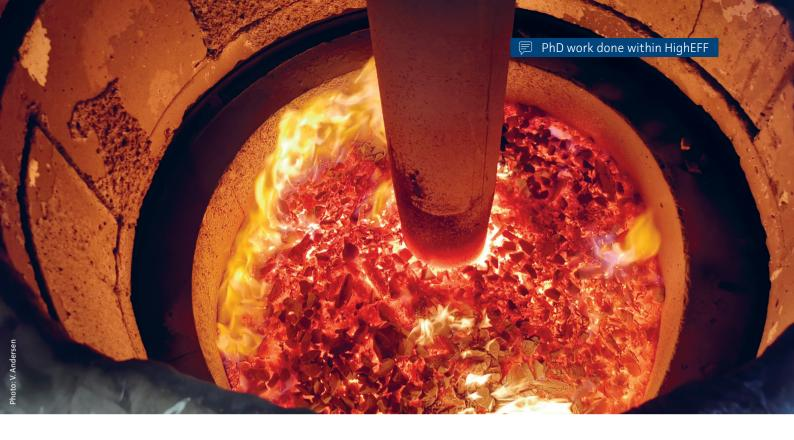
A look at the process of silicon production. Process gas burns over the raw materials in contact with air and recirculated exhaust gas.
