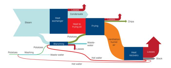
chip production line. Preliminary results indicate that the use of high-temperature heat pumps could reduce energy consumption by up to 60% and reduce  $CO_2$ emissions by up to 93%. This investigation represents a first phase in the study, and it is based on preliminary data received from Orkla. The considered processed data should be verified before investment costs are further evaluated.
