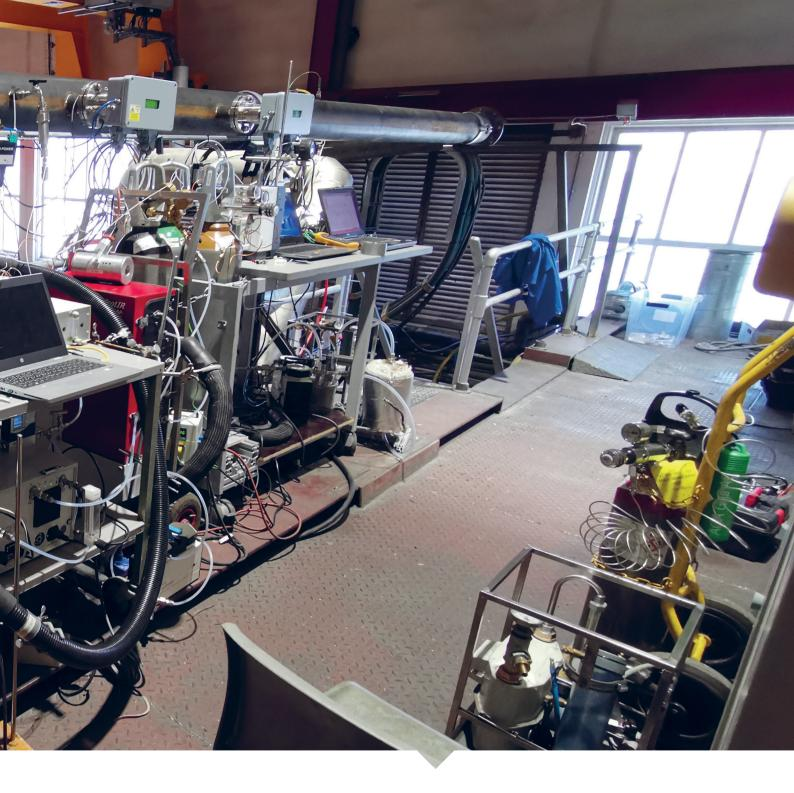
emissions and make  $CO_2$  capture easier for the silicon production process. The unique infrastructure built in Trondheim will be very valuable for future experiments and projects aiming at making metal production more sustainable in Norway and around the world. Above: Both the exhaust gas and the combustion air were analysed using two gas chromatographs, FTIR spectroscopy and LaserGas II instruments from NEO Monitors AS.
