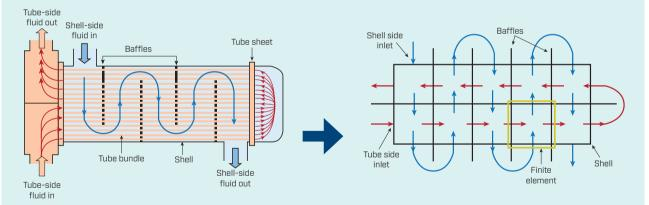
Discretization of a two-pass shell-and-tube heat exchanger
