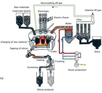
*Illustration that shows how recirculating off-gas can be done in the silicon production process. Illustration modified. Illustration: Halvard Tveit, Elkem (CC BY-SA 4.0).*
