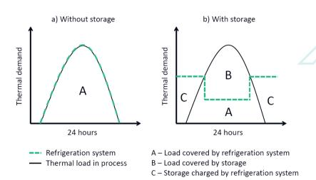
Figure 2: Operating a refrigeration system in a process a) without thermal energy storage b) with thermal energy storage.
