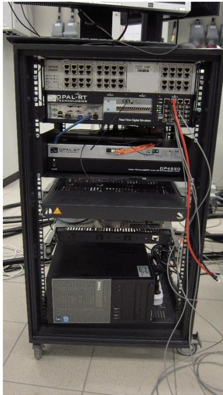
*Opal-RT Simulator to be used in the planned PhD experiments in the Norwegian Smart Grid Laboratory*
