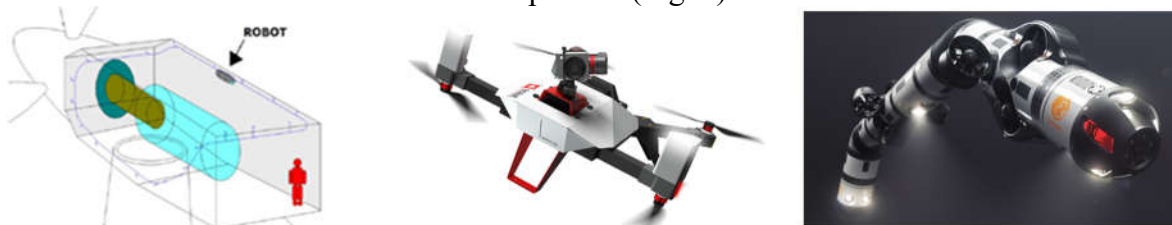
a) A robot for drivetrain inspection b) A remotely piloted Aircraft system for blade inspection c) Underwater snake robot vehicle
