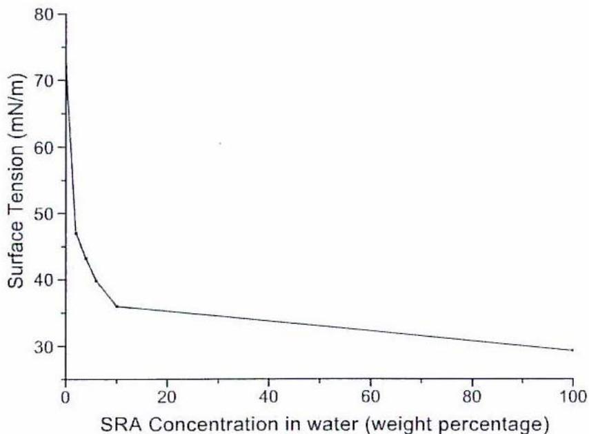
**Figure 10:** Effect of SRA on surface tension (Ronbing and Jian 2005)
