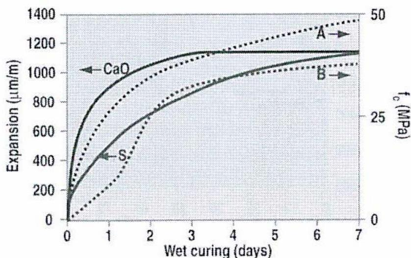
**Figure 9:** Restrained expansion and compressive strength ( $f_c$ ) for concretes with CaO or sulfo-aluminate (S) (Colleparidi et al 2005)
