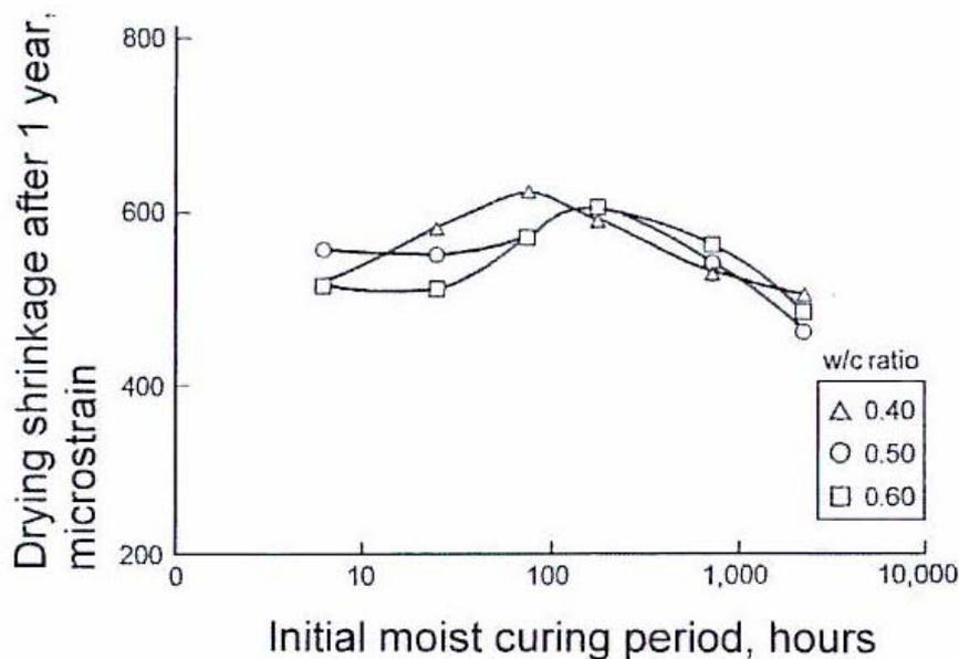
**Figure 8:** Effect of time of moist curing and water-cement ratio on drying shrinkage (Perenchio 1997)
