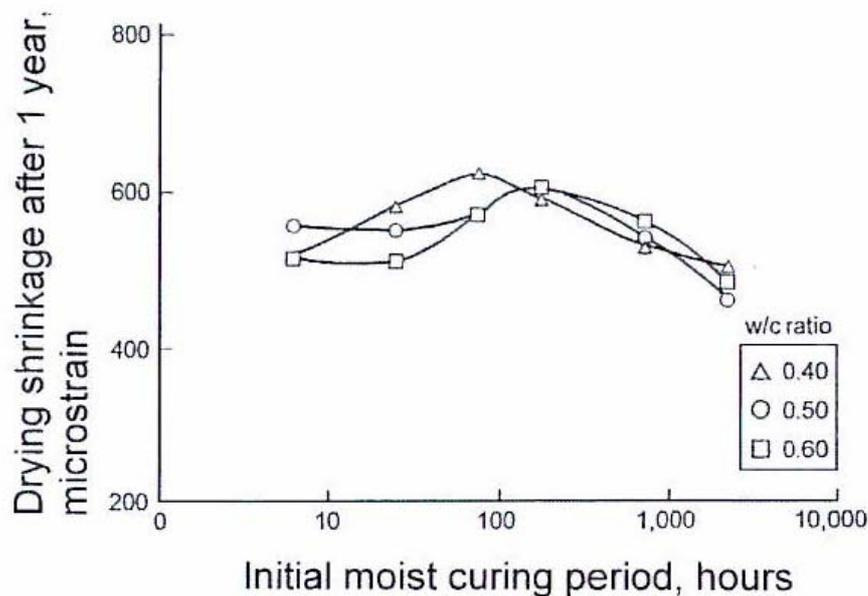
**Figure 8:** Effect of time of moist curing and water-cement ratio on drying shrinkage (Perenchio 1997)
