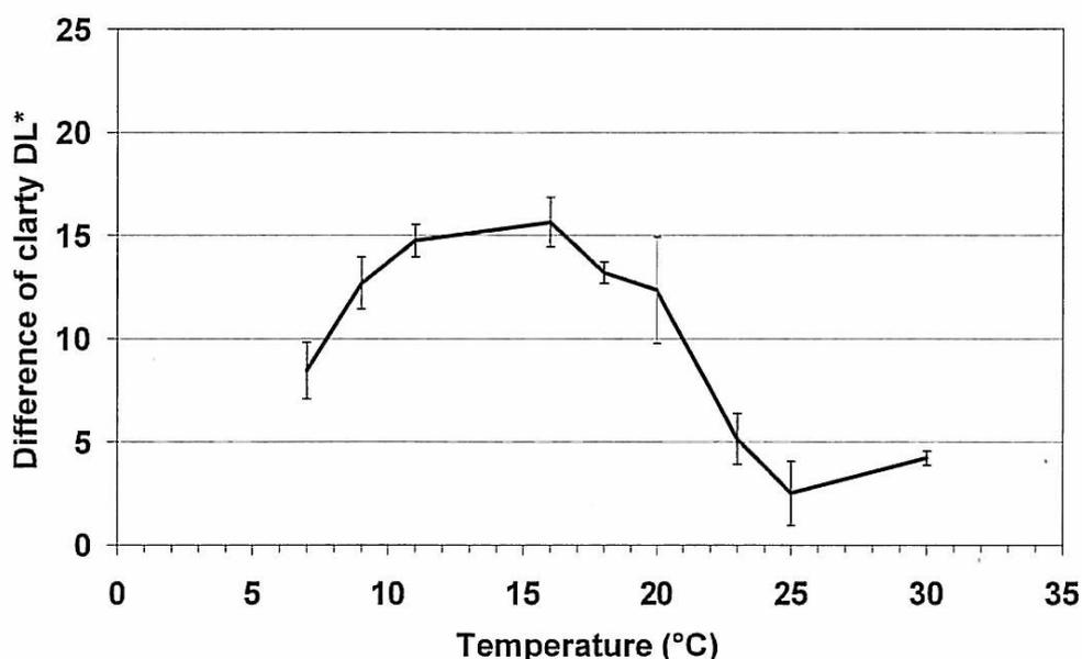
**Figure 2:** Influence of temperature on the formation of efflorescence (Delair et al. 2007)
