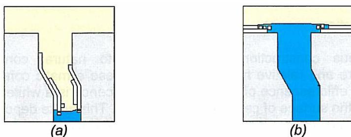
**Figure 3:** Influence of climatic conditions on salt precipitation. Image (a) shows precipitation within the pores as a consequence of fast drying, subflorescence. Image (b) shows precipitation of salts on top of the sample surface for slower drying rates, efflorescence (Delair et al. 2007)
