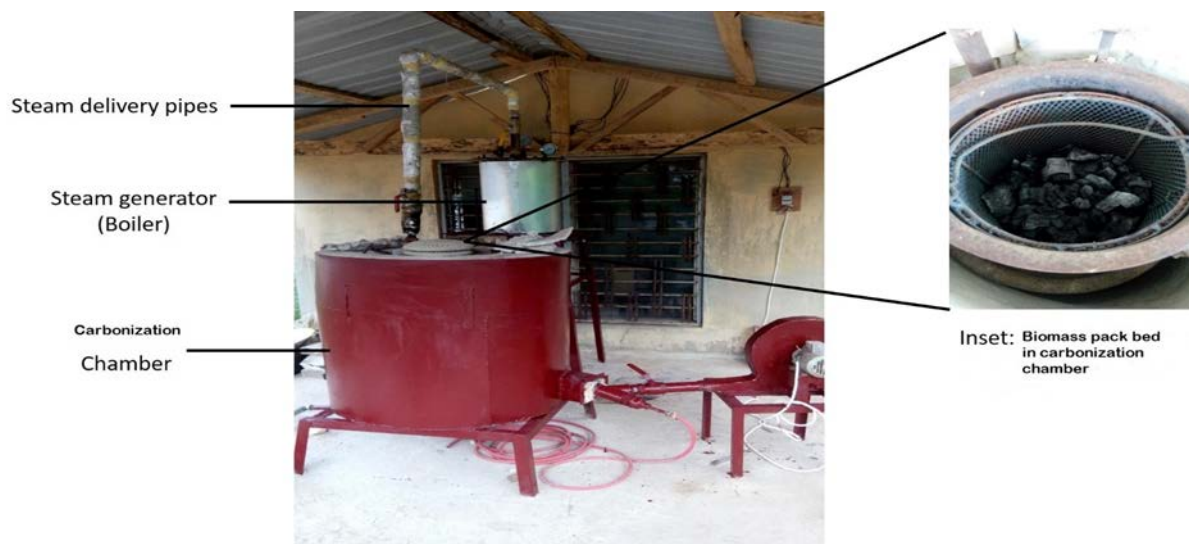
Figure 12: Picture of the carbonization rig fabricated for the temperature and time optimization study; Source: Authors
