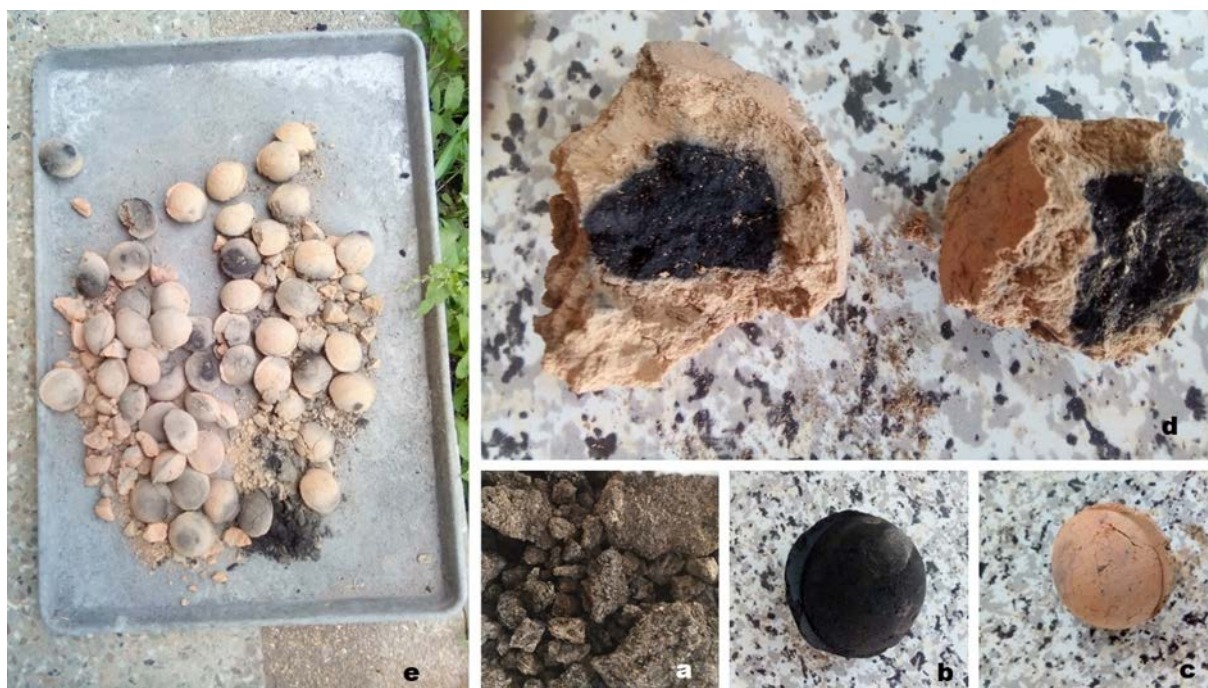
Figure 15: a) Sampled faecal sludge, b) biochar briquette from SSGL, c) sampled residual ash from WBT of b, d) Inner core of b showing unburnt carbon and e) Residual ash from WBT using Biochar briquettes from SSGL; Source: Authors
