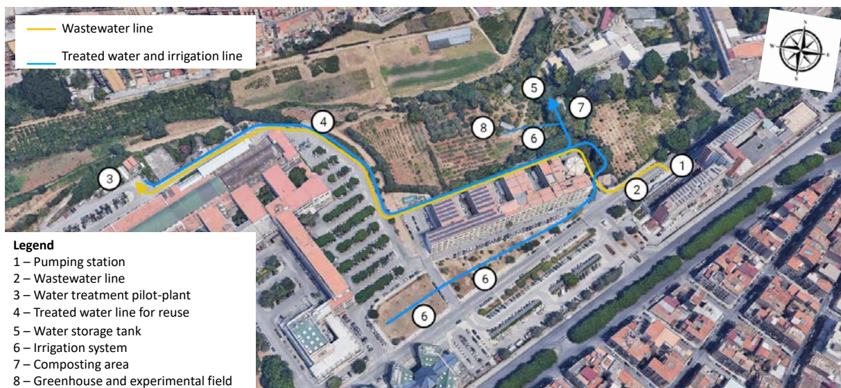
Figure 20: Panoramic view of Unipa Campus with the main elements of the reuse station
