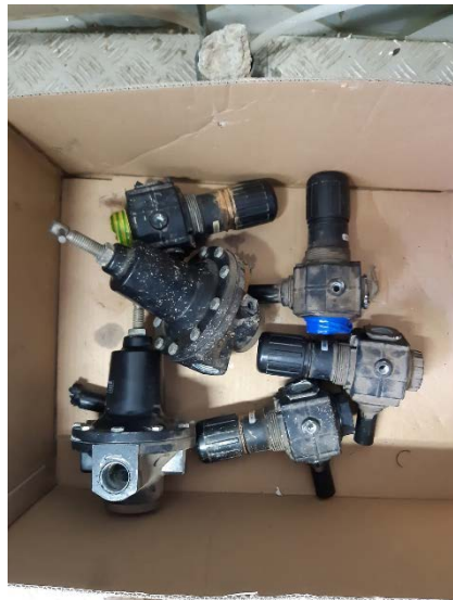
Figure 4: Disassembly of the pressure regulator
