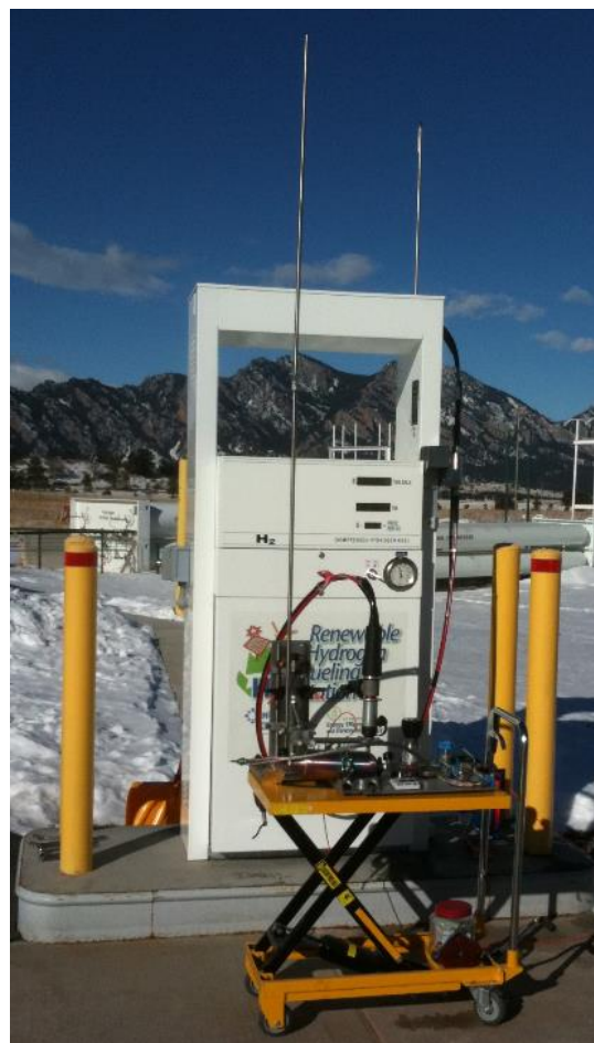
Figure 4: HQSA used by Smart Chemistry [4] (series sampling)
