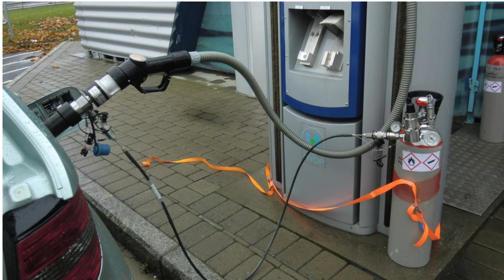
Figure 3: HQSA used in the HyCoRa project (parallel sampling)
