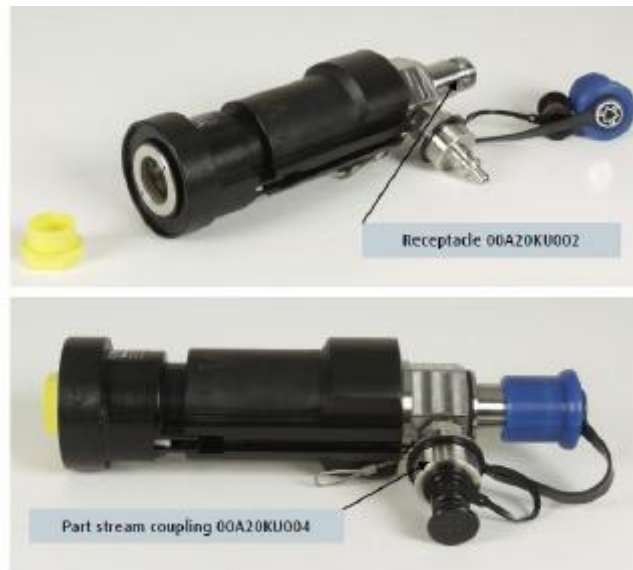
Figure 1: Tee adaptor used in parallel sampling
