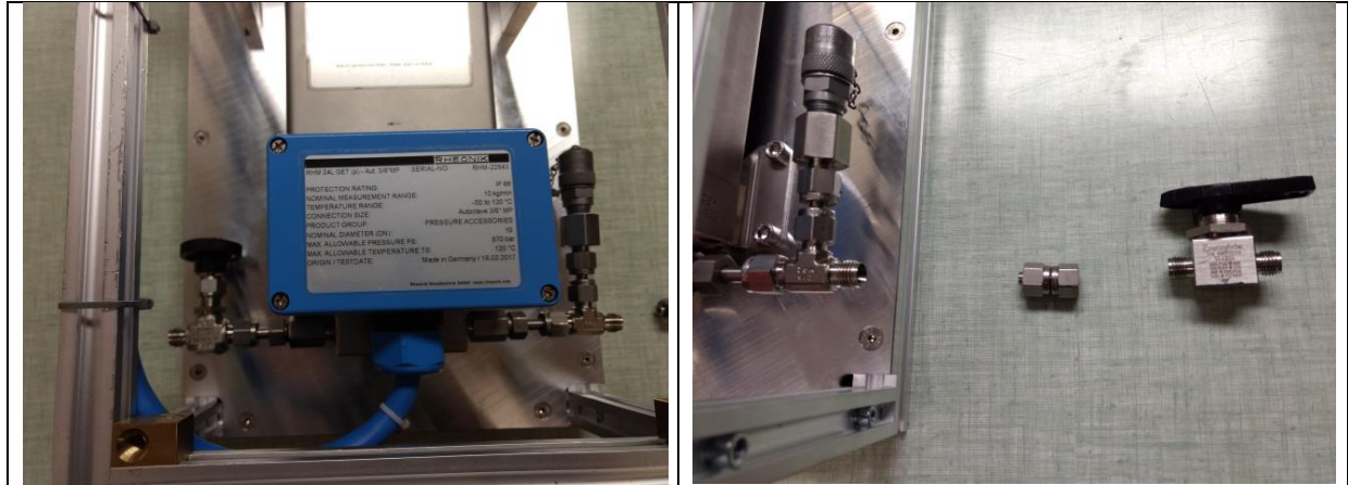
Figure 2: Left) CORIOLIS METER with needle valve and Minimes pressure fitting. Right) Ball valve with fitting. Flow direction is from right to left.
