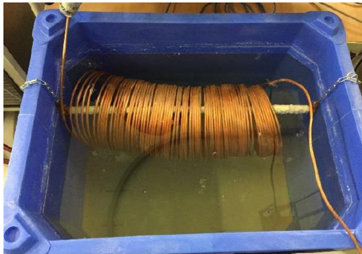
Figure 7: Passive heat exchanger used at METAS.
