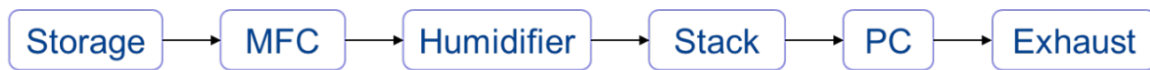
Figure 1 - Open-end test setup for PEMFC stack testing [4]. MFC is mass flow controller, PC pressure control.
