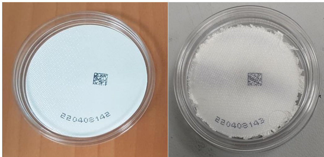
Figure 5: (left) PTFE glass fibre filter and (right) filter exposed to hydrogen
