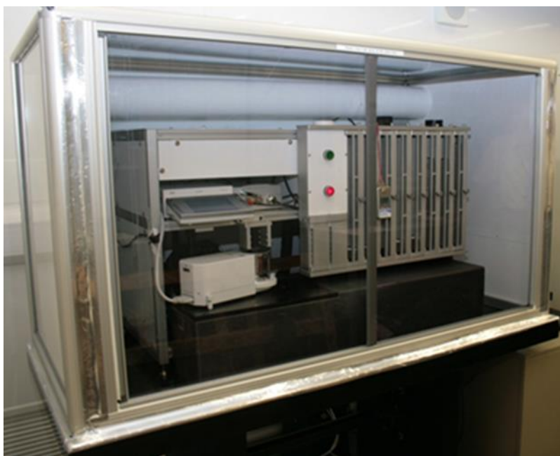
Figure 3: Chamber used for filter weighing at NPL
