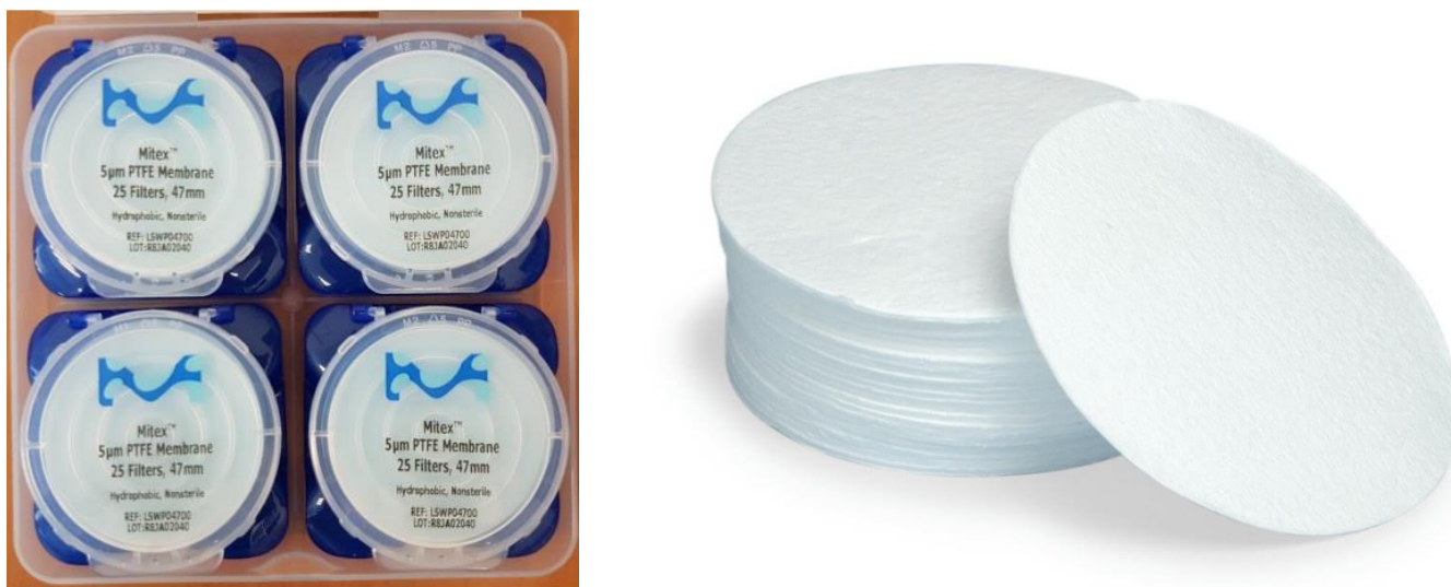
Figure 4: (left) PTFE porous filters in their packaging case and (right) quartz fibre filters [9]
