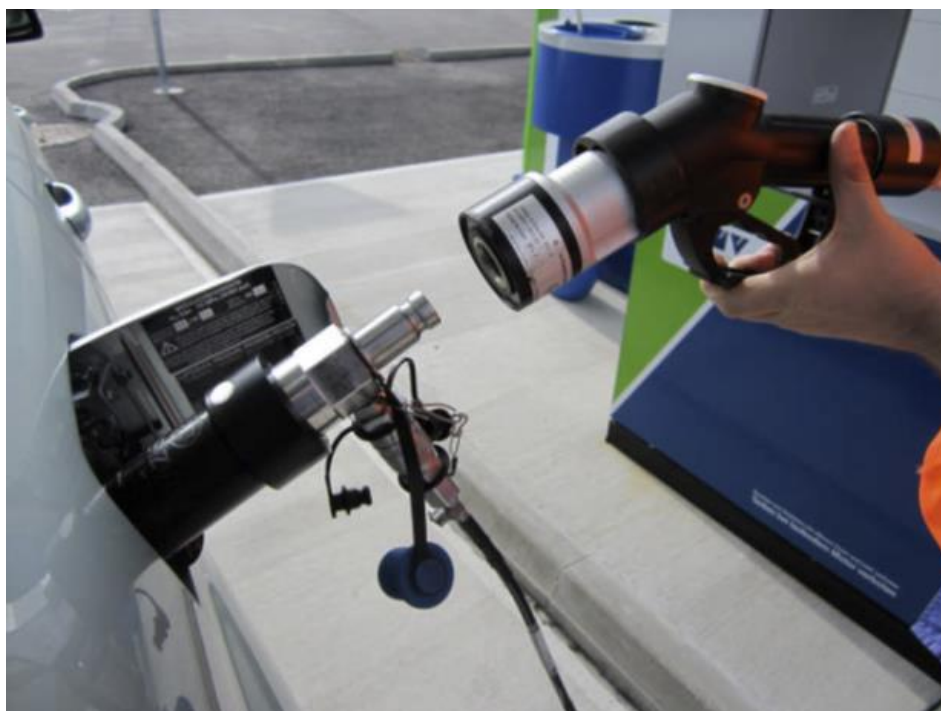
Figure 1: Installation of the Linde Qualitizer
