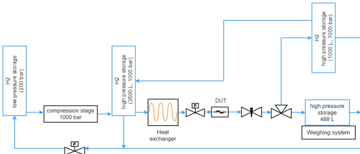
Figure 2: Piping and instrumentation diagram for the primary test rig for high-pressure calibration.
