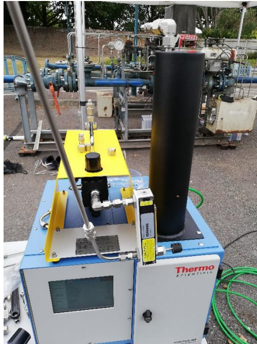
Figure 4: High Pressure Atomizer, H 2 Rotameter and TEOM instrument used during testing
