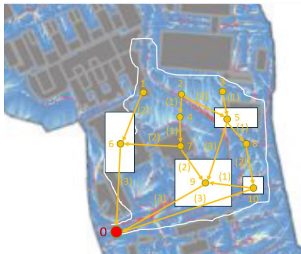
Figure 2: Example: Discretization of a catchment area into a network of nodes
