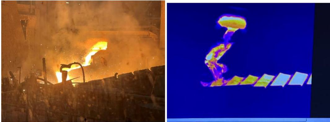
Figure 36 - Casting process as viewed from the control room (left) and through IR camera (right).
