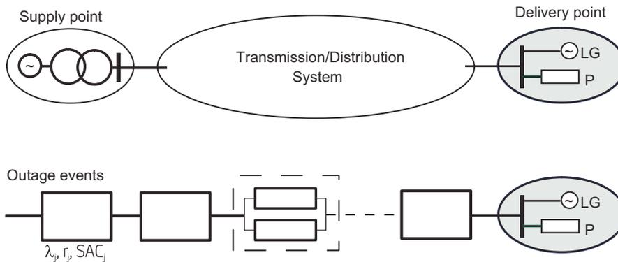
Fig. 4. Reliability model for a general delivery point based on minimal cut sets [38,39].
