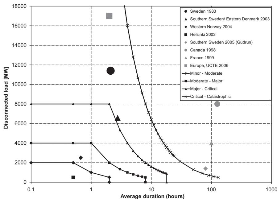
Fig. 2. Consequence diagram for the electricity supply, based on [32,33].
