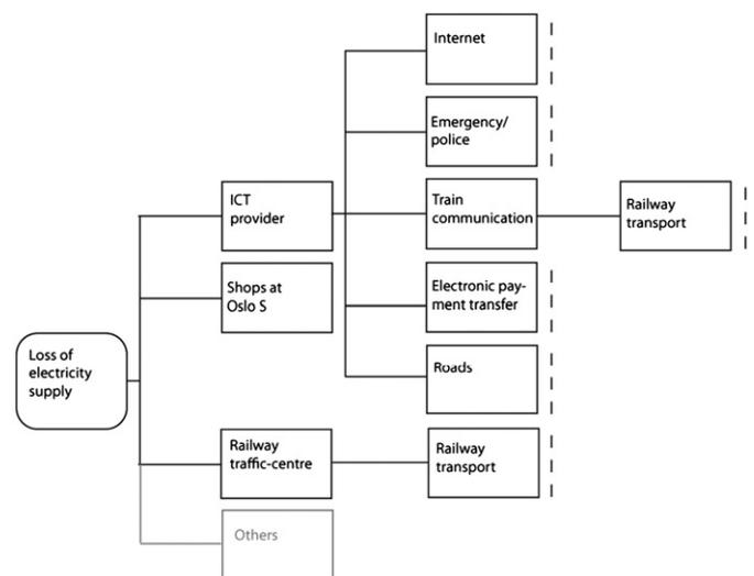
Fig. 7. Simplified cascade diagram for loss of electricity supply for the Oslo central station, based on [7]. The dashed lines indicate leaf-nodes.
