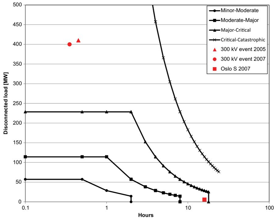
Fig. 6. Hazardous events in the electric power system in Oslo.
