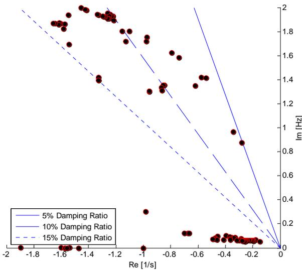
**Figure 7:** Electro-mechanical modes
