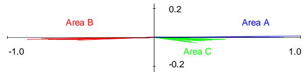
**Figure 8:** Mode shape plot of bus voltage angles for 0.93 Hz oscillatory mode
