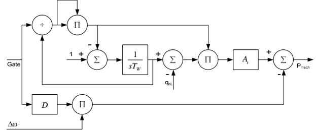
Figure 4: Hydro turbine system model
