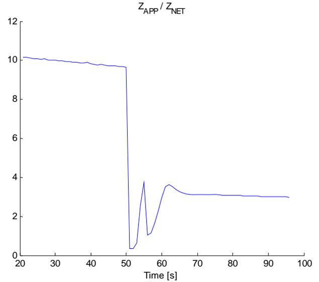
**Figure 11:** Impedance ratio between load and system at bus 109 during outage of transformers 109-111 & 109-112
