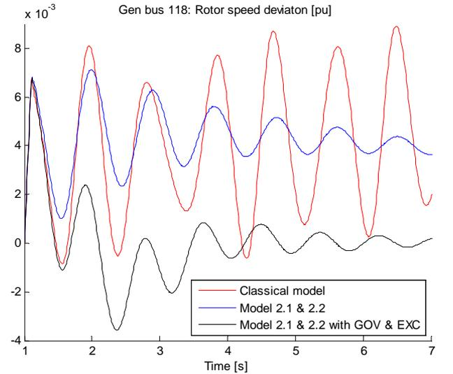
**Figure 1:** Rotor speed deviation of the machine at bus 118 for different dynamical models, when the system is exposed to a 3-phase fault on bus 119
