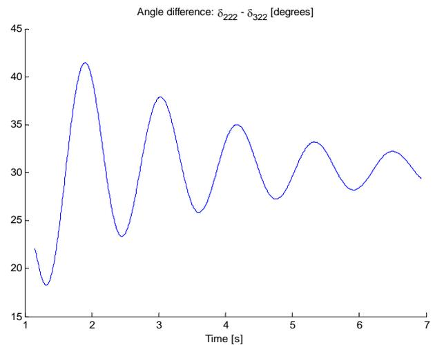
**Figure 9:** Voltage angle difference between bus 222 and 322
