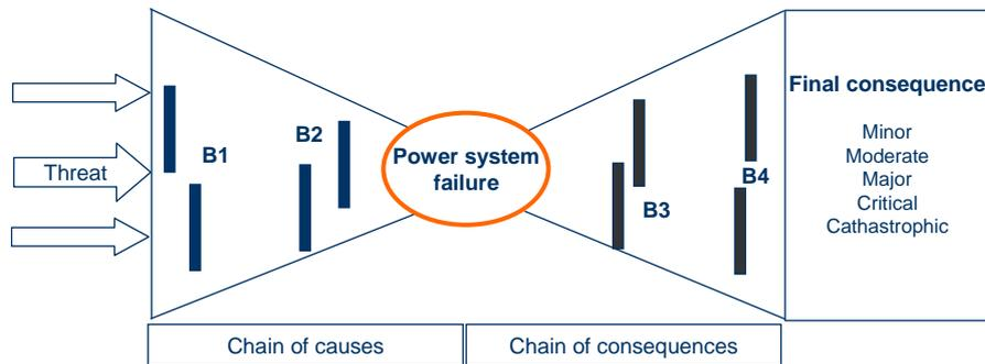
Figure 1 A Bow tie model for the event power system failure.
