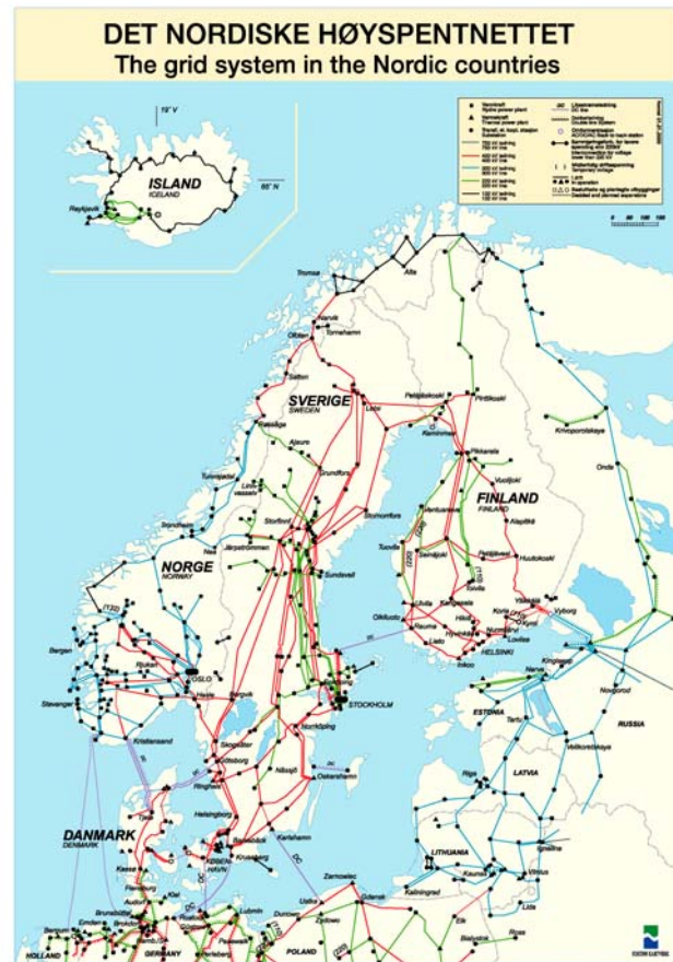
Figure 1. The grid system in the Nordic countries. Red = 400 kV, blue = 300 kV, green = 220 kV, black = 132 kV. 110 kV lines are not presented in this figure.
