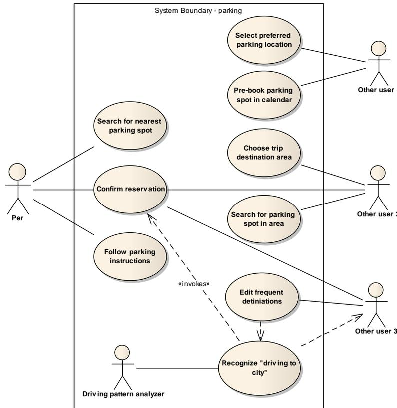
Figure 1 - Use case diagram for the parking scenario
