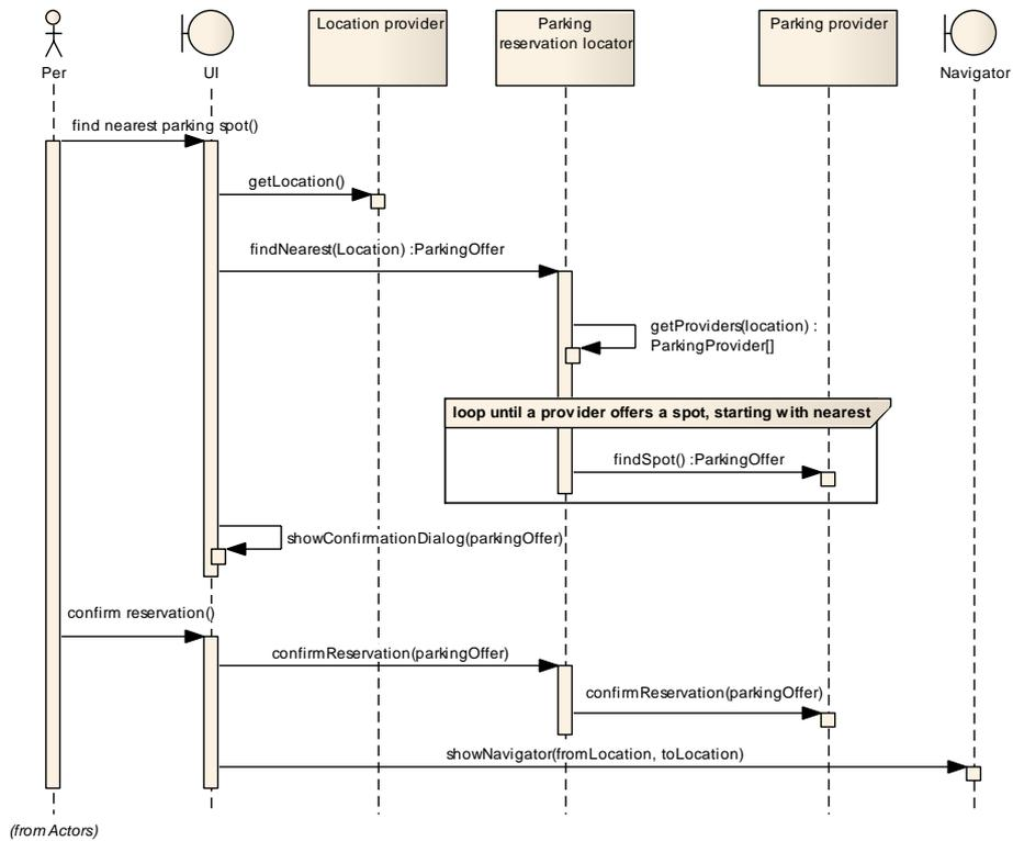
Figure 2 - Sequence diagram for the main parking activity scenario, finding nearest parking spot
