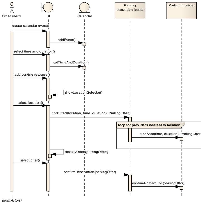
Figure 3 - Sequence diagram for pre-booking parking spot using the calendar
