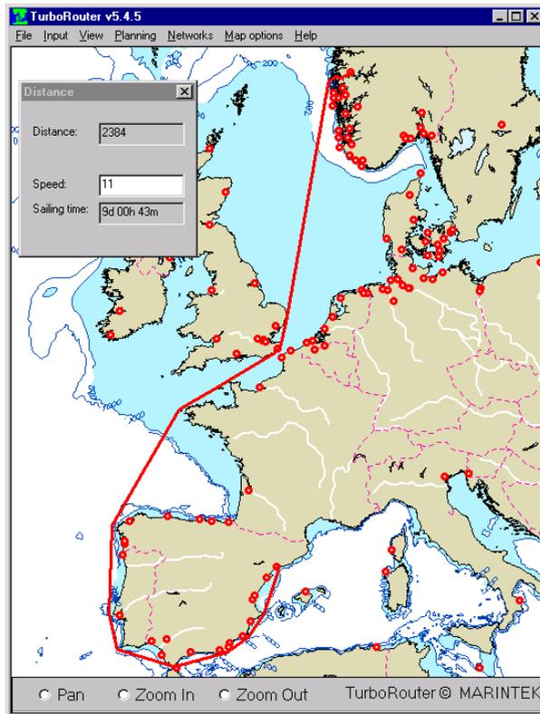
TurboRouter includes unique routines for calculating port-to-port distances. Instead of using static distance tables that are hard to keep updated, TurboRouter calculates the distance between any pair of ports. This is done by calculating the shortest (great circle) distance between the ports that does not intersect any land contours. Experience shows that the calculated distances are far within the requirements for this type of planning tool.
