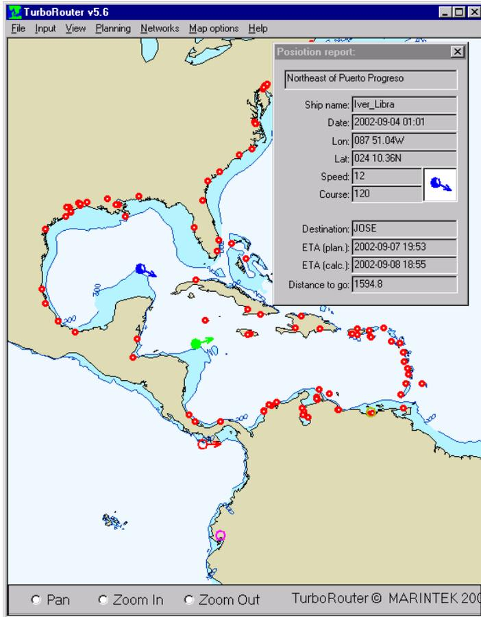
Satellite vessel position reports (provided by Pole Star) gives the planner an intuitive picture of fleet status. TurboRouter can calculate the distance and the sailing time from the ship position to the next port in the schedule. This function is also used for calculating updated ETAs. In this way, the planner can reveal deviations from the planned schedule at an early stage and make corrective decisions.
