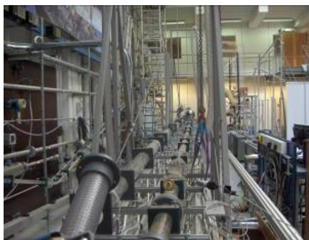
Multiphase flow test rig at the Department of Energy and Process Engineering, NTNU, (Photo : P. Klimantos)
