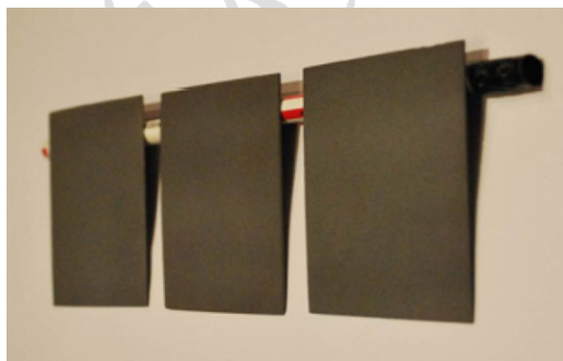
Figure 2 (online color at: www.pss-a.com ) Si wafers ( 65 \times 50 \text{ mm}^2 ) fabricated by thermal spray.
