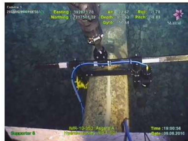
Picture 1: Tracerco Diagnostics Subsea Pipe Scan equipment
