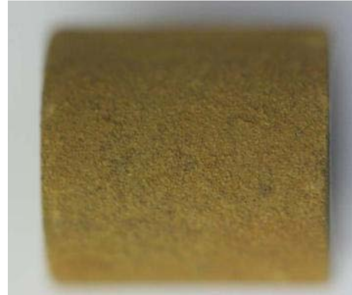
Pipeline steel with NO x corrosion product . Source: Doc 55430 Corrosion in dense phase CO 2 with small amounts of impurities- phase IV
