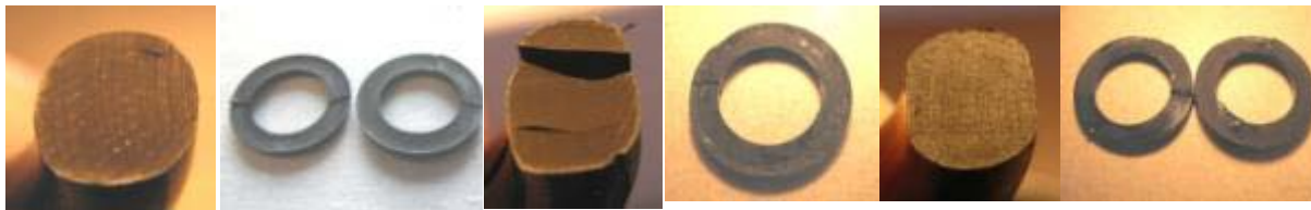
Test results for RGD with CO 2 . From left: FKM Terpolymer 90, Aflas 90, FKM (Viton ETP 90), HNBR 80, FFKM 90 and HNBR 95 ED (Carbon fibre and PTFE filled). Source: Doc 028012 Soft materials in valves for CO 2 transport in Offshore pipelines.
