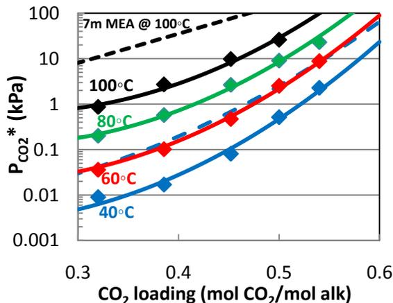
Figure 1: CO<sub>2</sub> solubility in 6.5 m β-alaK. Filled points: measured data. Solid lines: model prediction (Eq.1). Dashed lines: 7 m MEA model, Ref [2].
