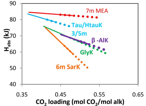
Figure 4: Heat of  $\text{CO}_2$  absorption predicted using regressed VLE model (Eq.1). Solid lines: coal operation range. Dotted lines: GTCC range. Red: 7 m MEA model, Ref [2].
