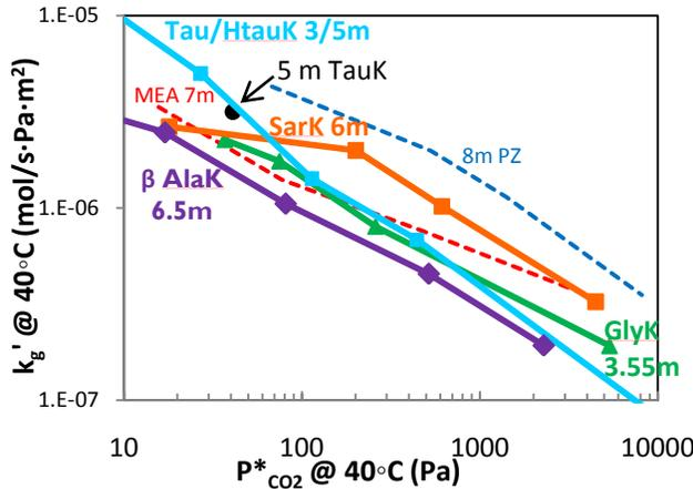
Figure 3: Measured absorption rates of amino acid solvents. Filled points: measured data. Dashed lines: 7 m MEA (red) and 8 m PZ (blue) results, Ref [2].
