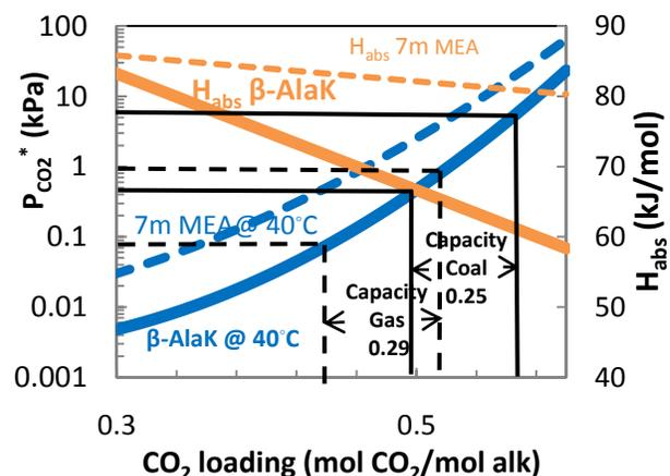
Figure 2: Cyclic capacity and heat of CO<sub>2</sub> absorption analysis for 6.5 m β-alaK. Dashed lines: 7 m MEA model. Ref [2].
