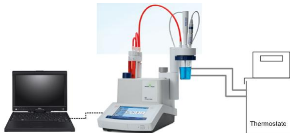
Figure 1. Set-up for potentiometric titration
