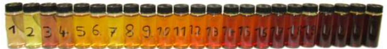
30% MEA degradation during 920 operating hours
