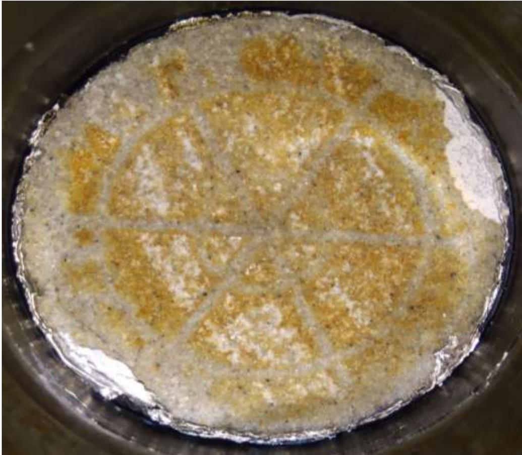
Core Outlet after CO<sub>2</sub> Injection
