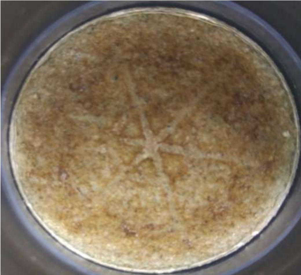
Core Outlet after CO<sub>2</sub> Injection
