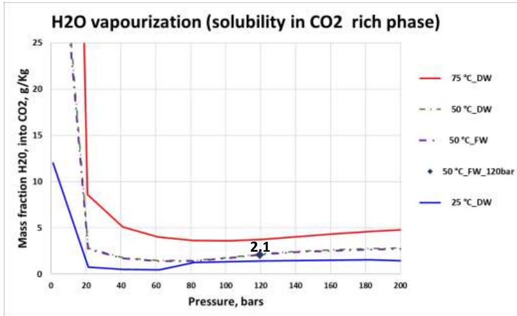
Evaporation of water at test condition
