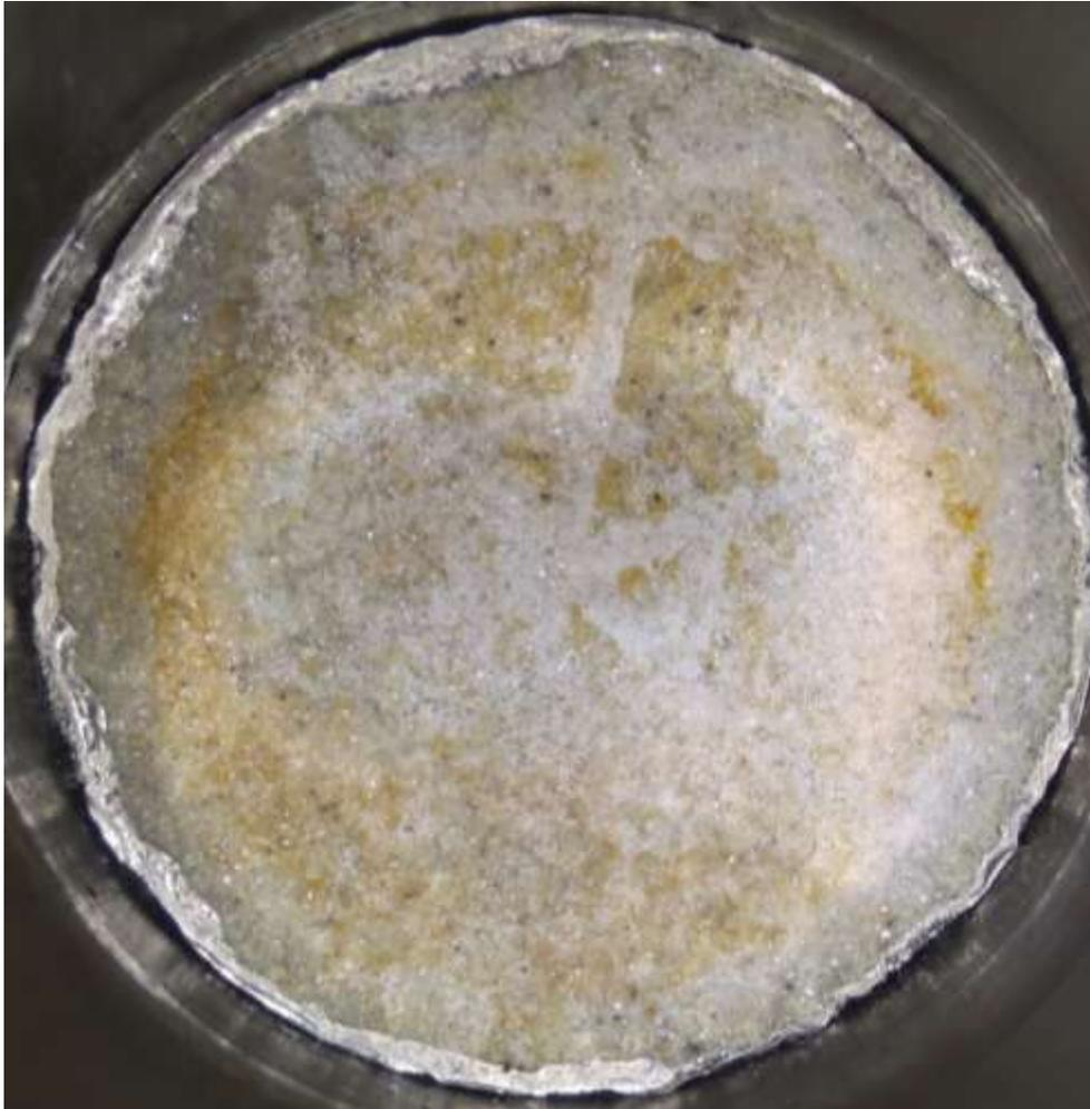
Core Outlet after CO<sub>2</sub> Injection
