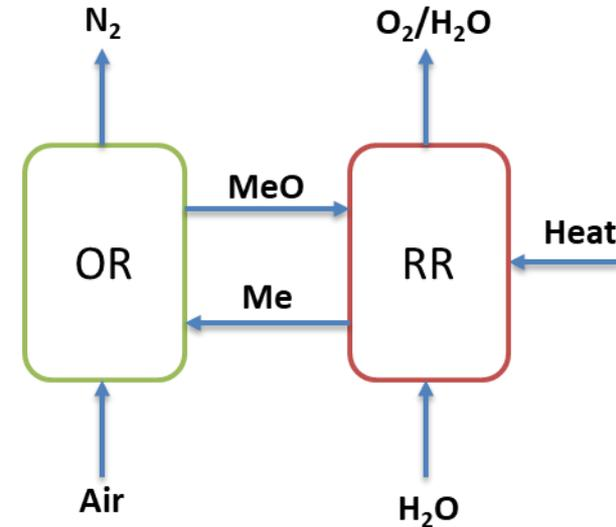
*Schematic of chemical looping air separation*
