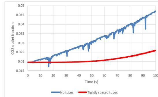
$\text{CO}_2$  mole fraction in the reactor outlet
