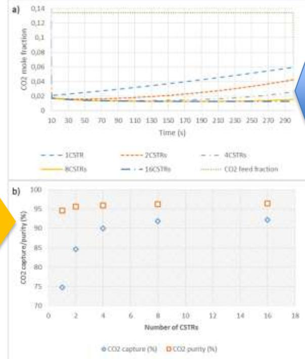
overall  $\text{CO}_2$  capture efficiency and purity
