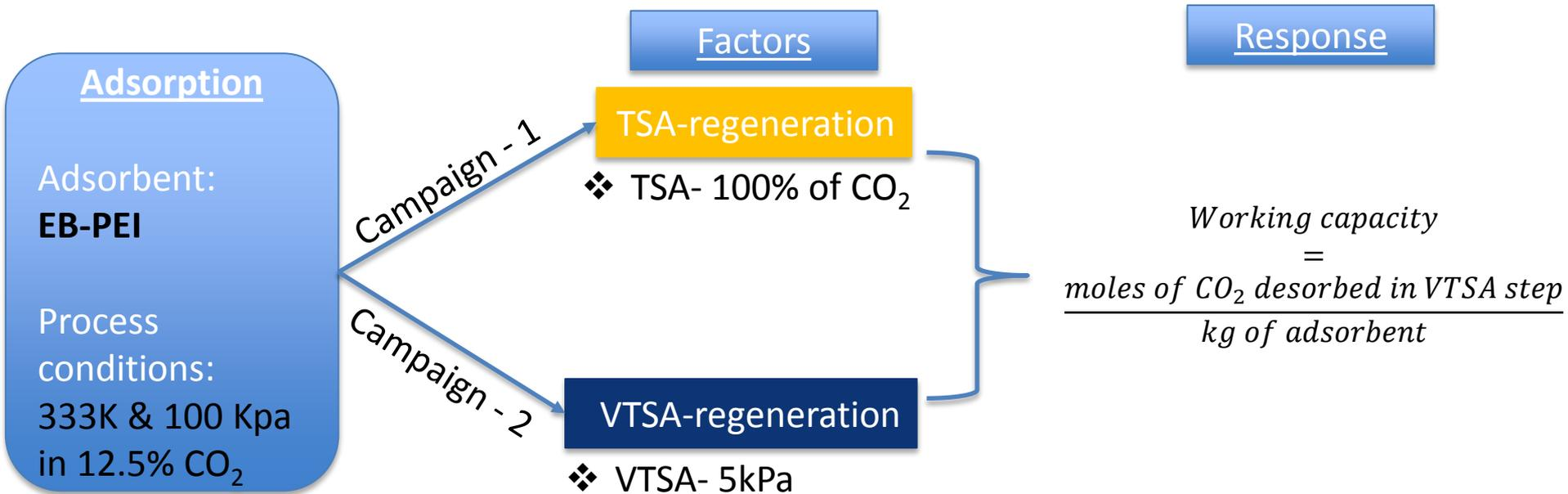
**EB-PEI** : 1,2-Epoxybutane functionalized polyethyleneimine supported on SiO<sub>2</sub> sorbent supplied by KRICT
