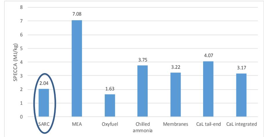
SPECCA: specific primary energy consumption per avoided CO<sub>2</sub> for the different CO<sub>2</sub> capture technologies
