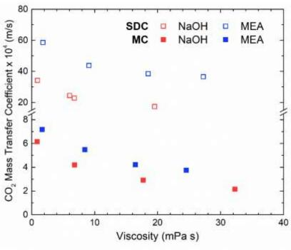
The CO<sub>2</sub> mass transfer coefficient drops with viscosity:
