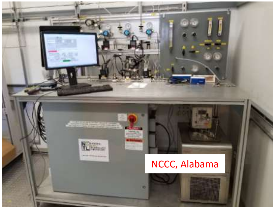
NETL's membrane flue gas test unit at the National Carbon Capture Center
