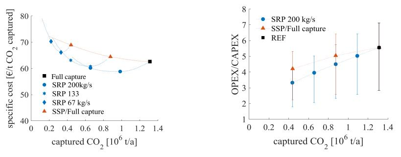
CO<sub>2</sub> concentration: 20 vol%; 200 kg/s Steam price 16 €/t; Electricity: 55 €/MWh
