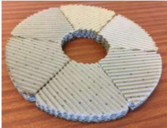
Montz structured packing – first prototype
