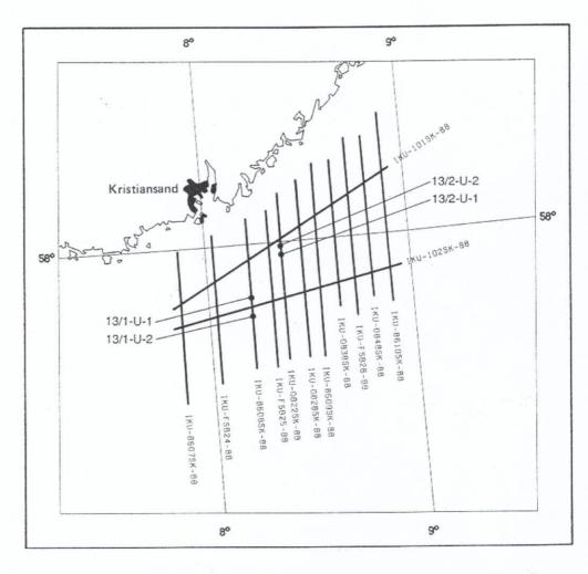
Approximately 670 km of shallow seismic was shot and four bedrock cores (370 m of bedrock samples) have been obtained.
