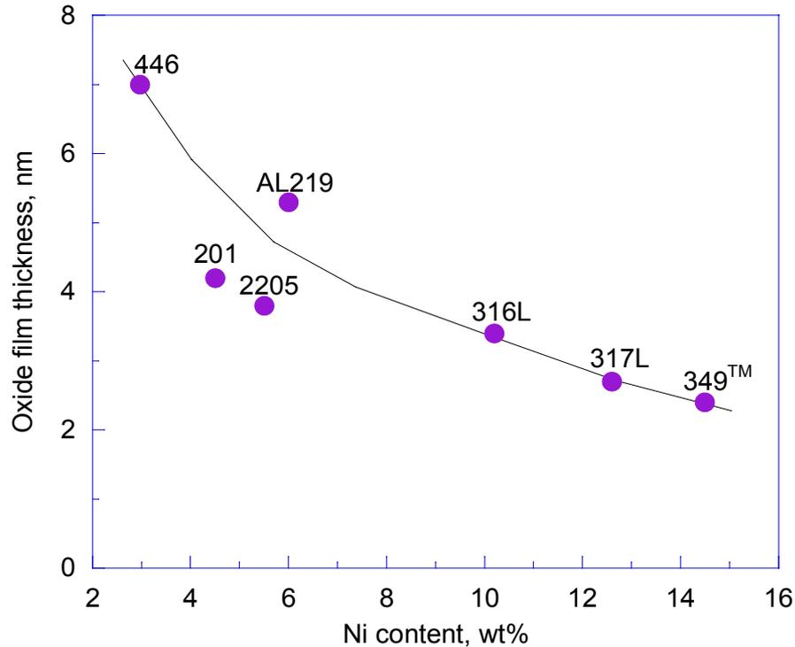
Dependency of air-formed oxide film thickness on the nickel content of stainless steels.
