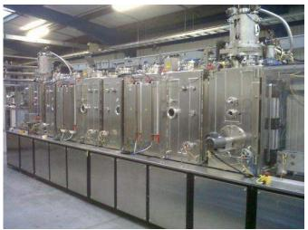
TCL in-line coating system for BPP to enable the coating of cleaned BBPs in semi-continuous process rather than a batch process, reducing process time and cost while increasing volume capacity.
