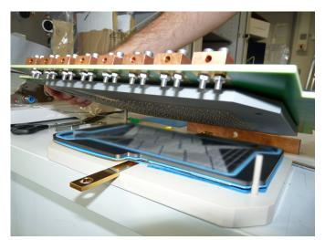
A segmented, automotive size graphitic test cell (LxWxH= 300x150x2 mm) and cell housing with compression unit and electrical cell contacts for the integration of the segmented cell.
