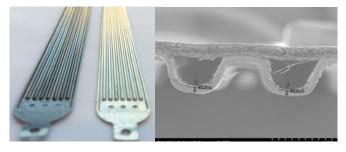
PVD coated and uncoated small scale BPPs (left), and combined GDL/BPP concept on stamped small size BPPs, where the GDL can be glued to the BPP with a non-conductive glue (right). SEM images for TiN-PANI coating with different coating time (below).
