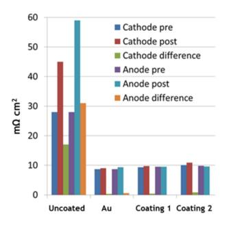
Status of best coatings after small scale in-situ AST, 100 hours cycling between OCV and 0.4 V.
